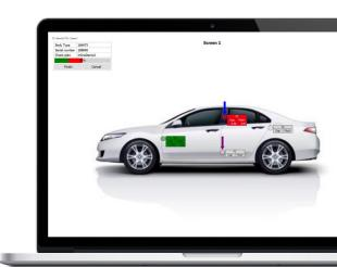
Inline is a Windows-based application designed to automate the inspection workflow. Inline provides live visualisations across multiple displays with clear instructions and overlays displaying measurement progress with pass/fail. Inline provides a faster and simpler way to use multiple GapGuns in a production environment.
