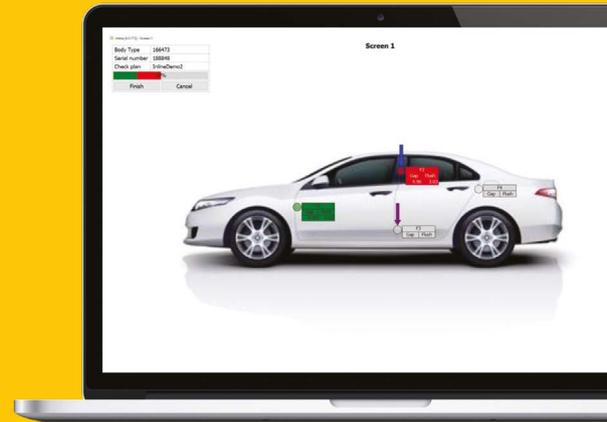
Inline is a Windows-based application designed to enhance inspection workflow on the shopfloor, when used together with the GapGun. It is a multifunctional piece of software: you can link multiple GapGuns together, view live results on different displays, as well as automate inspection plan selection and measurement reporting.
